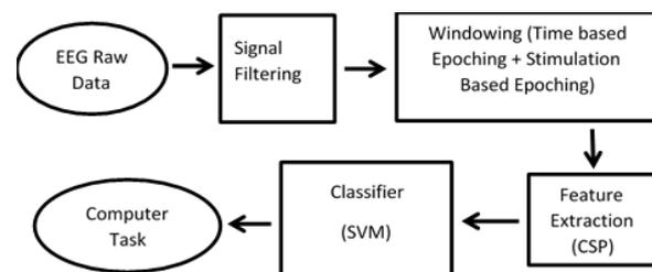
Figure 5. Block diagram of the BCI system
