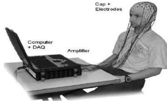
Figure 1. Components of a typical BCI system
